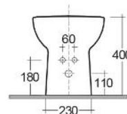
Dimensions: All dimensions in mm. Tolerance of vitreous china & fireclay items:  $\pm 5\%$  for below 200mm and  $\pm 3\%$  for above 200mm; for all other items tolerance  $\pm 1\%$ . Note: Due to a continuing development program to improve design and performance, the manufacturer reserves all rights to vary specifications without prior information. Please note accessories are for photographic use only.
